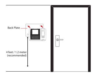
After determining the height of the terminal from the ground level and have made the relevant marks on the wall, drill the screws into the wall to hang the back plate.
